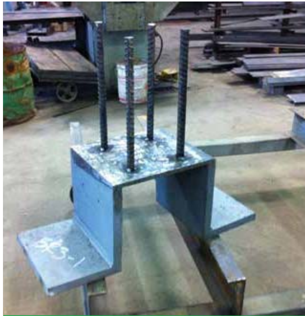
The column-to-column connector with saddles to carry glulam beams Courtesy: Fast + Epp
